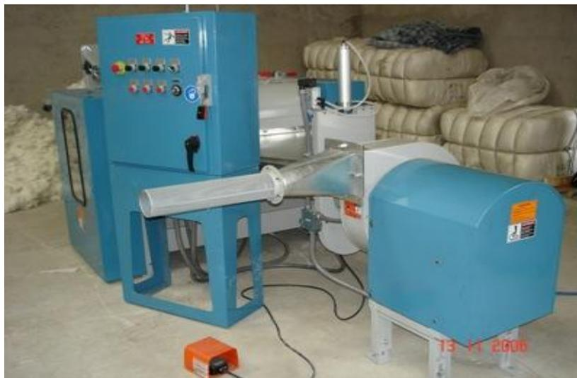
CCS offers many options such as multiple operator fiber filling stations, weigh system, timer feed controls, bar coding, variable speed motor drives, metal detection and humidification. Some custom systems are capable of producing as much as 3,000 pounds per hour. These systems generally include complete bale breakers that further reduce the labor requirement.
